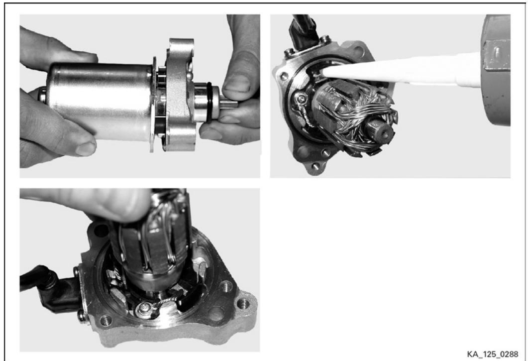
Figure 7.16: Electric starter disassembly
